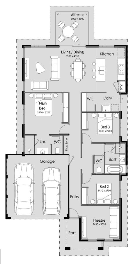
OVERALL WIDTH- 11.09m OVERALL LENGTH- 21.45m MIN BLOCK WIDTH- 12.50m MIN BLOCK LENGTH- 25m TOTAL AREA- 178.37m²
