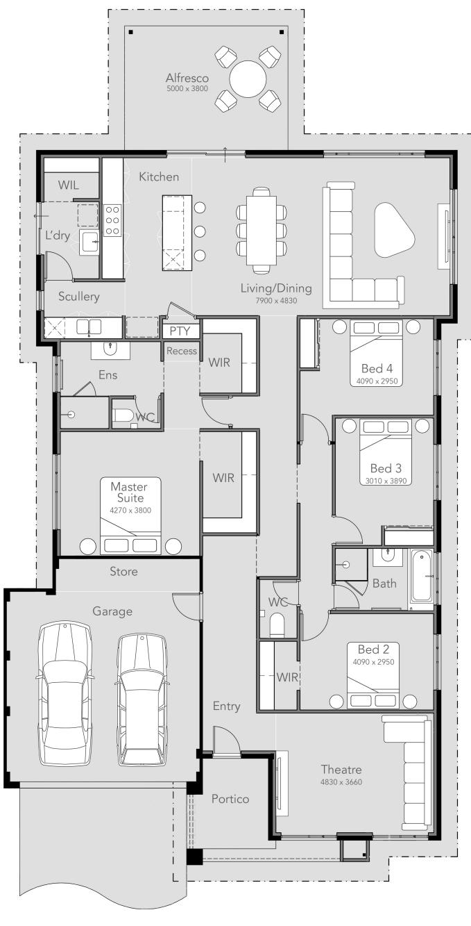
OVERALL WIDTH- 13.89m OVERALL LENGTH- 25.50m MIN BLOCK WIDTH- 14.94m TOTAL AREA- 281.03m<sup>2</sup>
